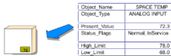
Figure 15: BACnet Objects with properties (capabilities, operation, related data)
