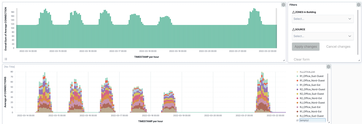
Figure 17 Result of Occupancy Prediction with continuous execution for a period of one week
