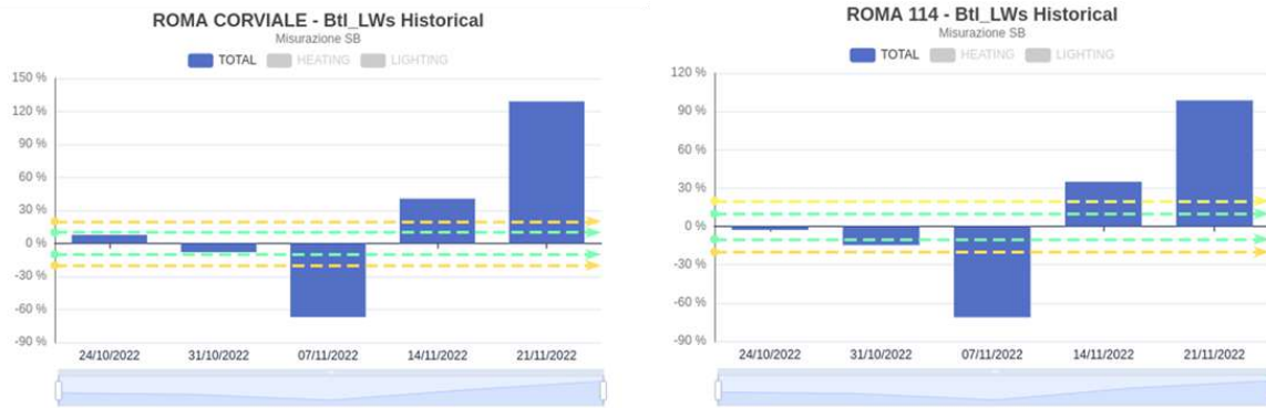
Figure 2: LLUC-3B_PI-01 KPI-03 Energy Consumption Gap of a building with itself during the short period
