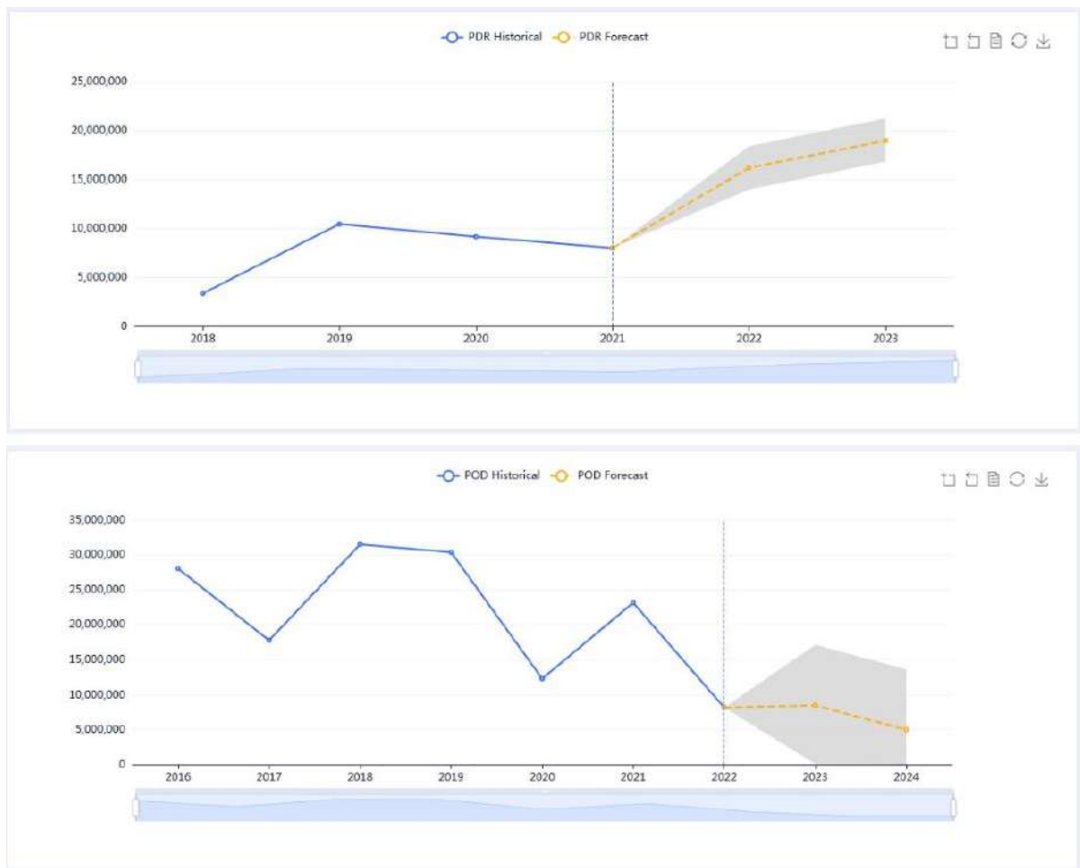
Figure 39 : Pilot 3b-ROM-03 – Forecasting dashboard: whole asset energy consumptions for Gas (PDR) and for Power (POD) meters. First algorithm PROPHET.
