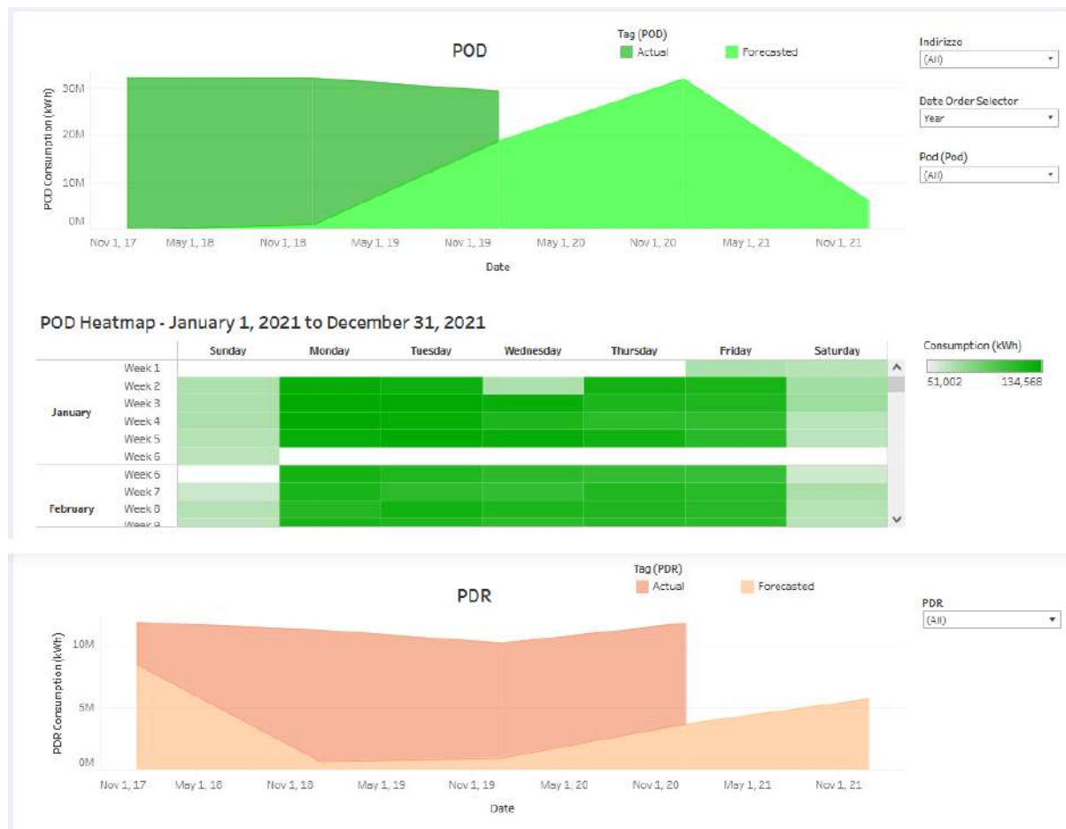
Figure 40 : Pilot 3b-ROM-03 – Forecasting dashboard: whole asset energy consumptions for Gas and for Power meters. Second algorithm DeepAR. A POD Heat map is also presented.
