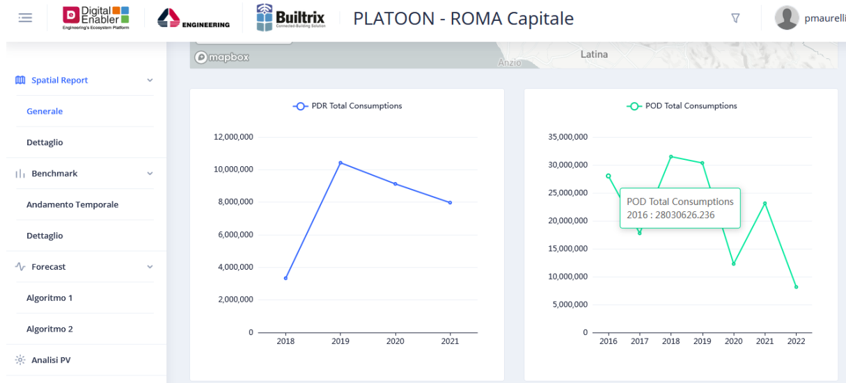
Figure 34: Pilot 3b-ROM-01 – Spatial Reporting dashboard: overall energy consumptions from Gas Meters annual data and Power Meters annual data, for the whole analyzed asset. The same can be done for clusters of buildings based on several selection criteria.
