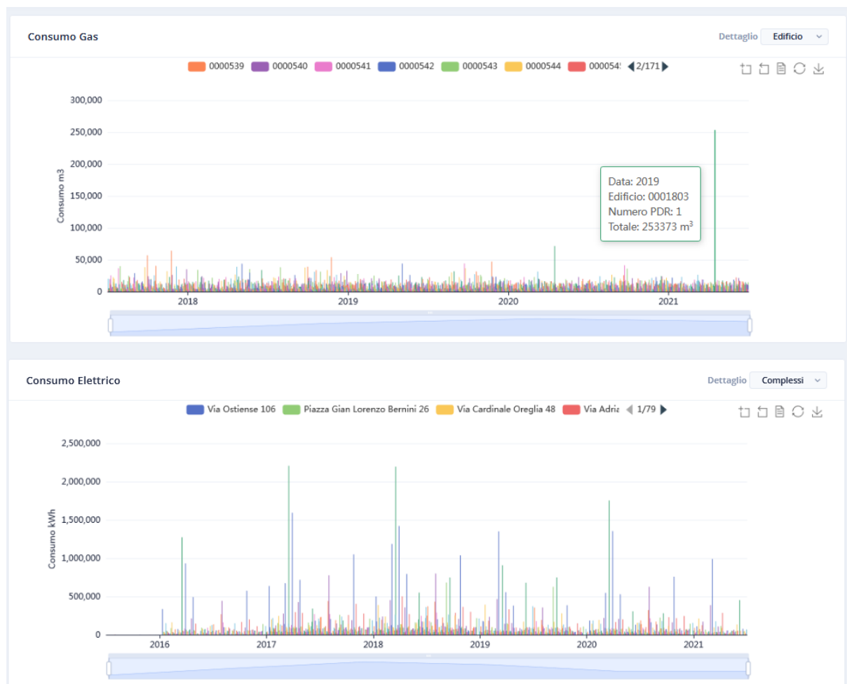
Figure 36: Pilot 3b-ROM-02 – Benchmarking dashboard: building energy consumptions compared year by year; note the anomaly Gas metering for building n.1803 on 2021
