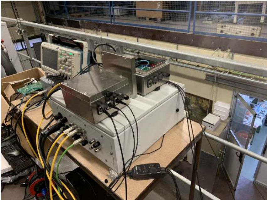
Figure 10: Picture of the setup that is used to acquire current measurements on the three phases of the generator.
