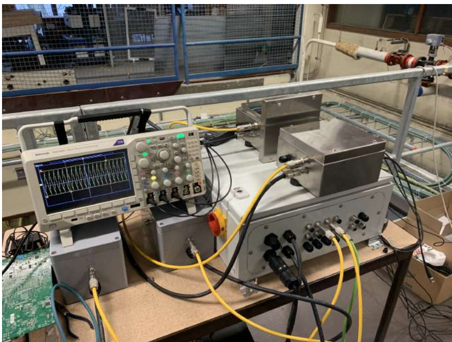
Figure 11: Picture of the setup that is used to acquire current measurements on the three phases of the generator.
