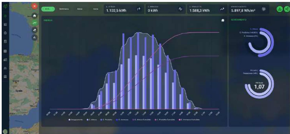
Figure 49: Venera IoT Dashboard – PV energy generation
